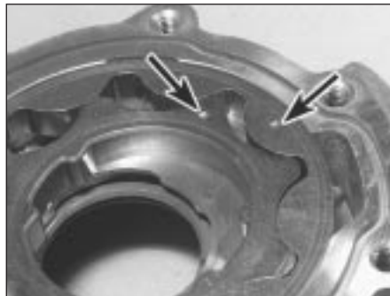
15.4 Inner and outer rotor matchmarks (arrowed)
