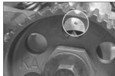
3.6b Camshaft sprocket timing mark aligned with the TDC mark on the front face of the cylinder head
